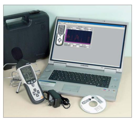
This sound level meter measures the acoustic pressure. The purpose is to determine and control the noise pollution in the working area, in conformity with the norm CEI61672-1 Class 2.
